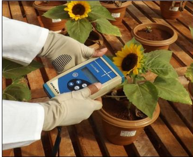
Figure 3. Ornamental sunflower plants indirect chlorophyll content readings with a chlorophyll meter.
