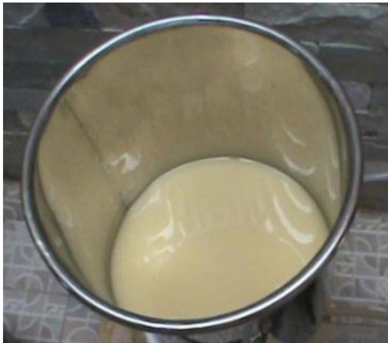
Figure 1. Preparation of fermentable wort in steel vat, up to 30 liters of wort.
